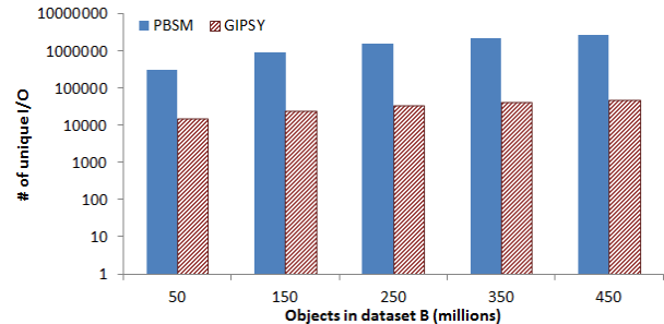
Figure 12: Number of I/Os (logscale) as a result of one spatial join, building mesocircuits.
