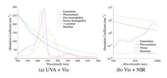
Figure 3. The spectral absorption coefficients curves for the skin chromophores included in our model from 300nm to 1000nm.
