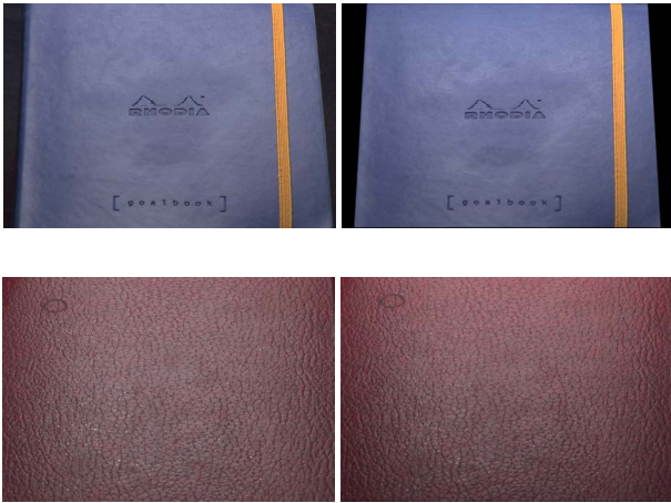
Figure 13: Comparison of photographs (left) to Mitsuba2 renderings (right) created using the SVBRDF maps estimated by our method
