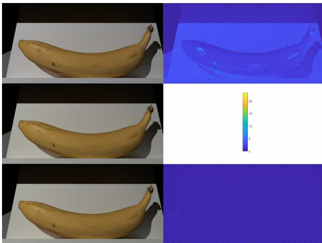
Figure 11: Comparison of full ground truth spectral rendering under D65 illumination (middle row), with a RGB rendering using for the illuminant the RGB values corresponding to D65 (top row), and rendering with spectral upsampling of RGB using our optimized Gaussian basis (bottom row). The result of our spectral upsampling is indistinguishable from the reference rendering, while color differences in the RGB rendering are clearly visible.
