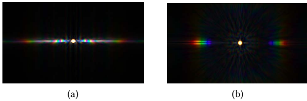
Fig. 19. Diffraction patterns rendered from grating measurements using bokeh photography. (a) CD. (b) Blazed diffraction grating (ThorLabs).
