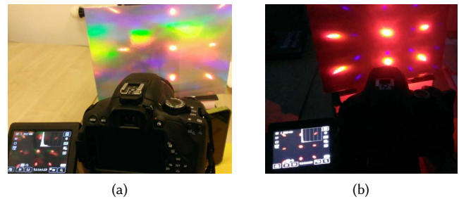
Fig. 5. (a) Measurement setup shown with the house lights switched on. (b) An LED flash illuminates the sample with a red spectral filter for measurement of the diffraction pattern.
