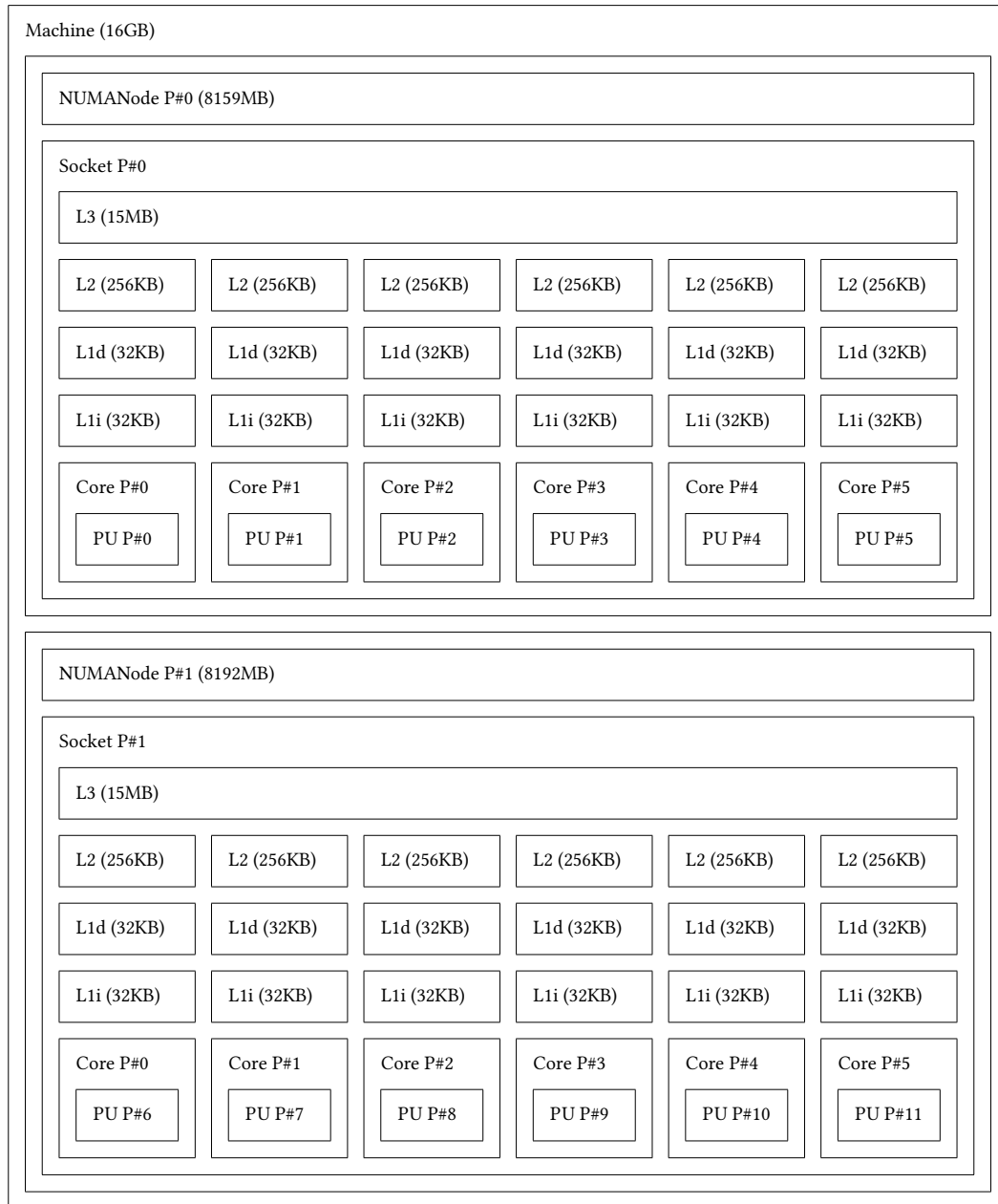
Figure A.2.: The CPU cores and cache on the CX1 node, as reported by lstopo .
