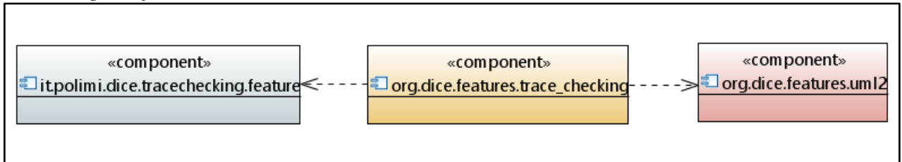
Figure 10: Components and dependencies diagram for Trace Checking Tool.
