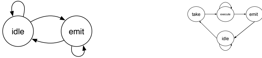
(a) Finite automaton describing the states of a bolt (b) Finite automaton describing the states of a bolt
