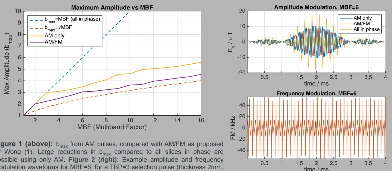
**Figure 1 (above):**  $b_{\max}$  from AM pulses, compared with AM/FM as proposed by Wong (1). Large reductions in  $b_{\max}$  compared to all slices in phase are possible using only AM. **Figure 2 (right):** Example amplitude and frequency modulation waveforms for MBF=6, for a TBP=3 selection pulse (thickness 2mm, gap 18mm). AM achieves 87% of the amplitude reduction compared with AM/FM but the latter requires rapid frequency modulation as shown
