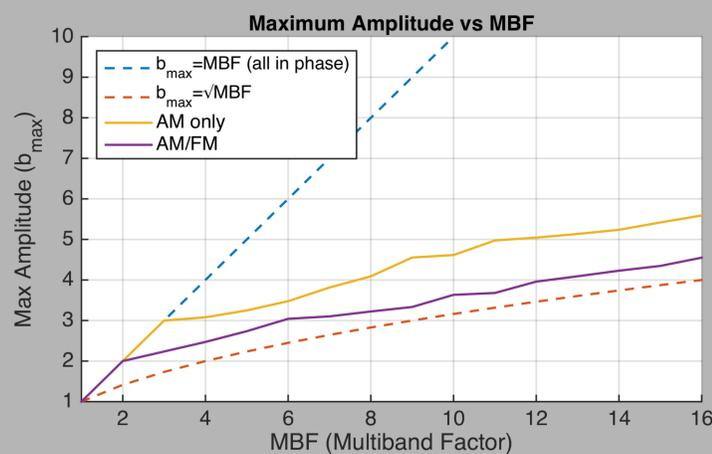
**Figure 1 (above):**  $b_{\max}$  from AM pulses, compared with AM/FM as proposed by Wong (1). Large reductions in  $b_{\max}$  compared to all slices in phase are possible using only AM. **Figure 2 (right):** Example amplitude and frequency modulation waveforms for MBF=6, for a TBP=3 selection pulse (thickness 2mm, gap 18mm). AM achieves 87% of the amplitude reduction compared with AM/FM but the latter requires rapid frequency modulation as shown
